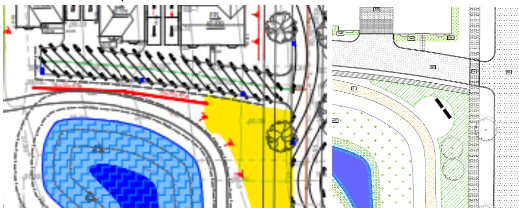
The retaining wall in this location has been removed, however the levels plan still does not reflect proposed and existing contours, thus landform details remain unclear. This must be addressed in order to confirm the suitability of the scheme.
