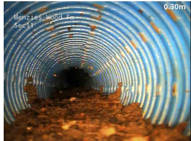
2, 00:00:09, 0.30 m Settled deposits, fine, 25% cross-sectional area loss
