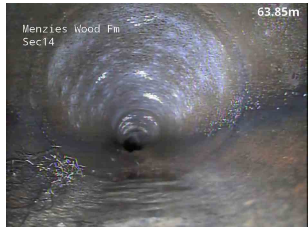
8, 00:03:39, 64.00 m Roots, fine at joint
