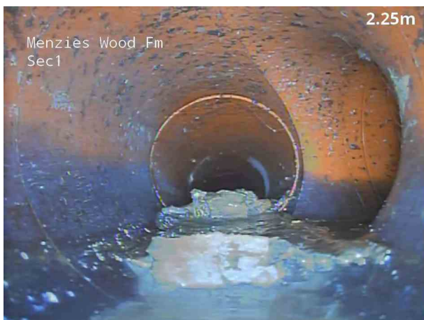
5, 00:00:48, 2.40 m Settled deposits, hard or compacted, 15% cross-sectional area loss
