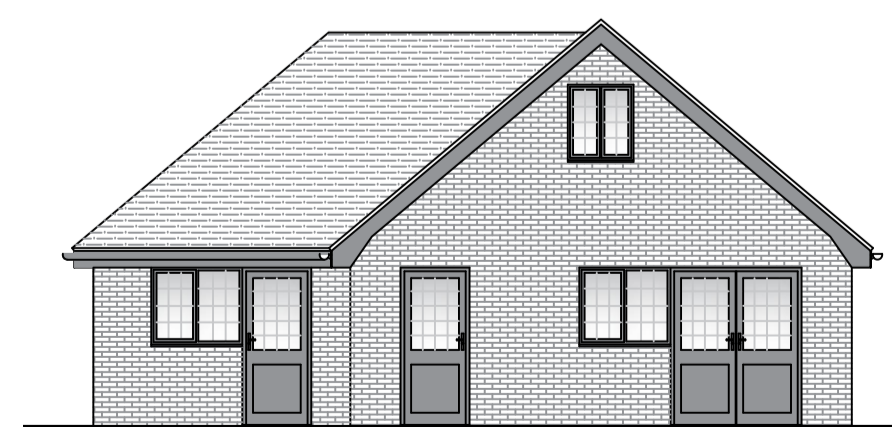
Garage - Existing Rear Elevation (Scale 1:100)
